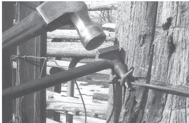
**Staple puller has a long point at one end with a flat driving plate behind it. You position point between post and staple and use a hammer to drive it in.**
