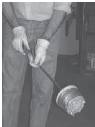
**Homemade magnetic pickup tool discharges its load with one easy movement of handle.**
