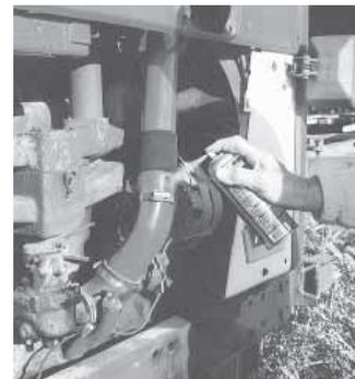
**Marley sprays ether into a hole drilled into the intake air pipe leading to carburetor. Then he slides sleeve down over hole.**
