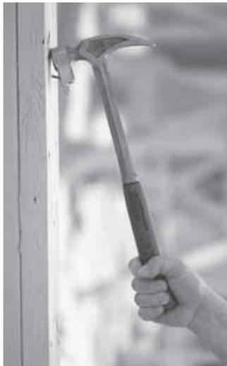
**Hammer's front-mounted claw pulls 12 to 20-penny nails with no need to flip the hammer over.**
