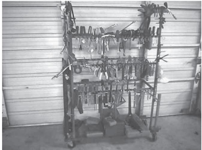
Homemade portable cart is made from welded-together angle iron with pegboard hooks welded to horizontal cross members.
