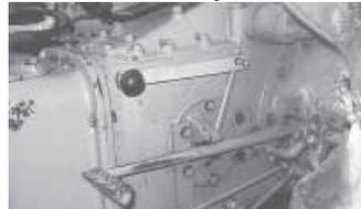
lever is located too far down and too far back. To solve the problem, I clamped a 12-in. length of strap iron on top of the lever and mounted a ball knob on one end of it. The knob extends much farther forward than the original lever, and brings it right up near the driver where it's easier to reach."
