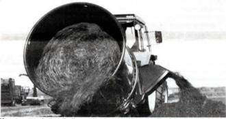
Hopper rotates hydraulically, moving feed over knives and out side discharge chute.
