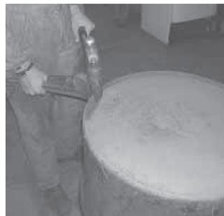
cause I didn't know what kind of material the barrel originally contained. To solve the problem, I closed the jaws of a pipe wrench just enough to get the jaws over the folded rim of the barrel. Then I used a big hammer to hit the back side of the top jaw until the jaw punched through the barrel. Once I made that initial hole through the rim, I was able to tip the wrench on its side and take half bites
