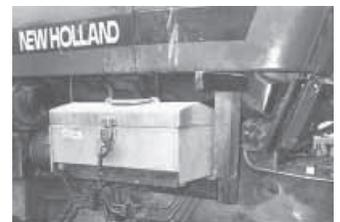
Ford New Holland tractors - a 3930, TN 70DA, and 2600. The factory toolboxes on these tractors are either too small or located too far off the ground to see into them without having to climb into the cab. With my add-on toolboxes I always have enough tools on hand, and they're easy to get at. They also provide extra room for bolts, fencing materials, and other miscellaneous stuff."
