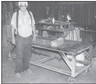
to make it big enough. That's what Charles did when he used a full 4 by 8-ft. sheet of 5/16-in. steel for a table top when making a rolling work table. He built a sturdy wood frame below and added locking caster wheels. He says the heavy steel top takes a beating and is plenty big for all kinds of repair work.
