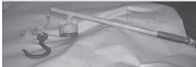
Tool consists of a metal cup that fits over end of drill and an 18-in. long metal handle that hinges on cup. A hook is welded to end of handle to hold a piece of chain.
