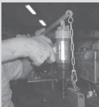
While holding the drill with one hand, the operator uses his other hand to pull down on the handle to provide leverage.
