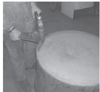
cause I didn't know what kind of material the barrel originally contained. To solve the problem, I closed the jaws of a pipe wrench just enough to get the jaws over the folded rim of the barrel. Then I used a big hammer to hit the back side of the top jaw until the jaw punched through the barrel. Once I made that initial hole through the rim, I was able to tip the wrench on its side and take half bites
