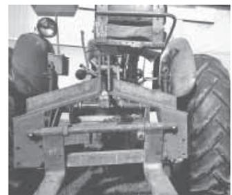
Dietz mounted a pair of forks on a toolbar carrier that mounts on his tractor's snap coupler hitch and extends under tractor.
