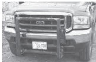
When blower is removed, truck-mounted subframe looks like a heavy duty push bar.
