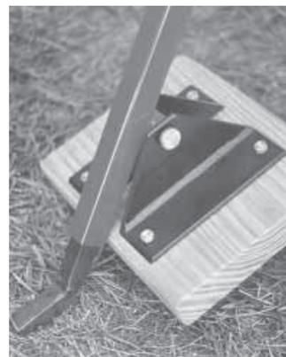
To remove a shrub, you insert the hook under shrub’s root system, then step down on platform and pull back on handle at the same time.
