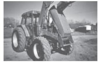
Light guard is made of two triangular steel plates that bolt to sides of tractor's front-end loader frame.
