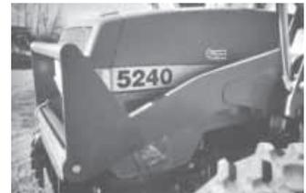
A 2-in. heavy-wall pipe is welded between the tops of the plates. "We've never broken a light since I put these shields on," says inventor John Tesch.
