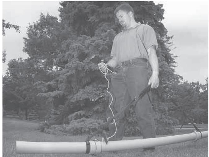
Hand held data reader is connected to sensors inside an 8-ft. long pipe. It works because soil contaminated with household waste has a higher electrical conductivity.
