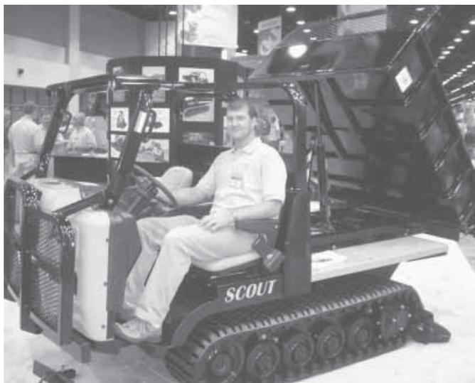
The new ASV Scout, with its 4,000-lb. bed capacity and 5,000-lb. towing capacity, is designed for much heavier work than most utility vehicles.
