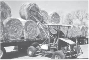
Leonard Sjoberg built his "Blazer loader" using the chassis and running gear off a 1970's 4-WD Chevrolet Blazer. "It works great for loading round bales onto trucks."
