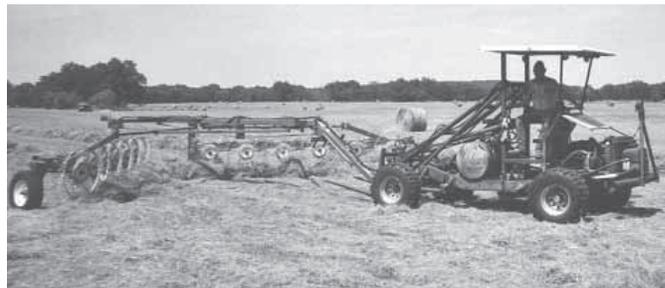
Loader can also be used to pull this 20-ft. wide V-rake, or a side delivery rake.
