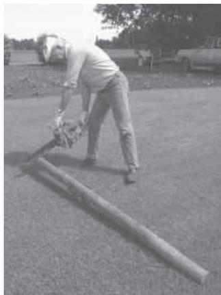
Using a special "fork", Mel Primrose is able to hold the end of a log about 4 in. off the ground as he cuts it.
