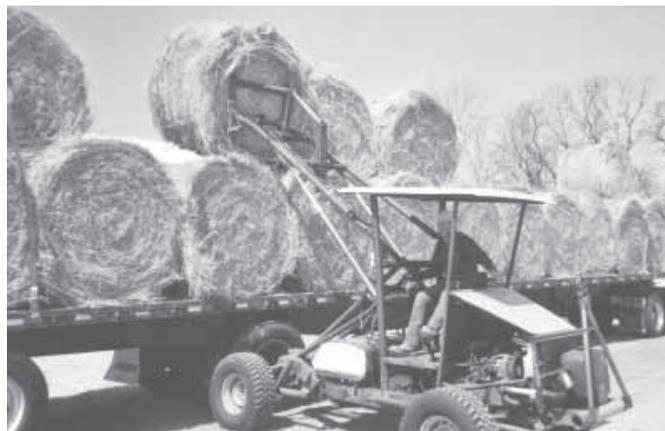
Leonard Sjoberg built his "Blazer loader" using the chassis and running gear off a 1970's 4-WD Chevrolet Blazer. "It works great for loading round bales onto trucks."
