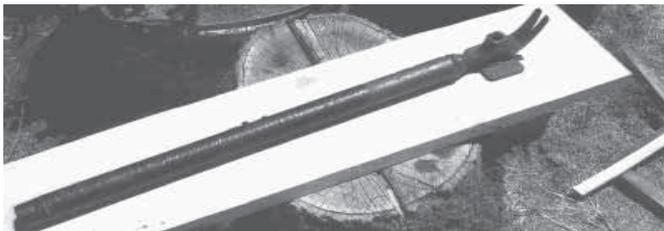
Fence stretcher was made by welding a length of pipe to a hammer head, then welding a flat plate to the top.
