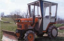
Using 1-in. steel tubing, sheet metal and plexiglass, Glenn Dawson built this cab for his Kubota B5200 4-WD, 13 hp tractor.
