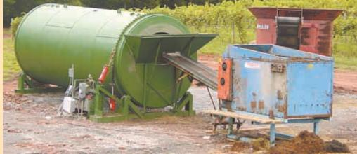
Large fuel and water tanks are turned into "continuous fill" compost tumblers, driven by electric or hydraulic motors.
