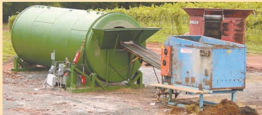
Large fuel and water tanks are turned into “continuous fill” compost tumblers, driven by electric or hydraulic motors.
