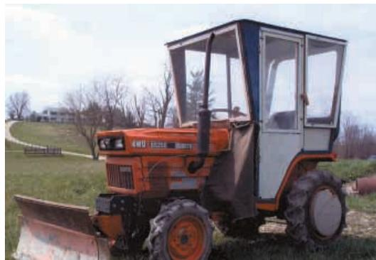
Using 1-in. steel tubing, sheet metal and plexiglass, Glenn Dawson built this cab for his Kubota B5200 4-WD, 13 hp tractor.
