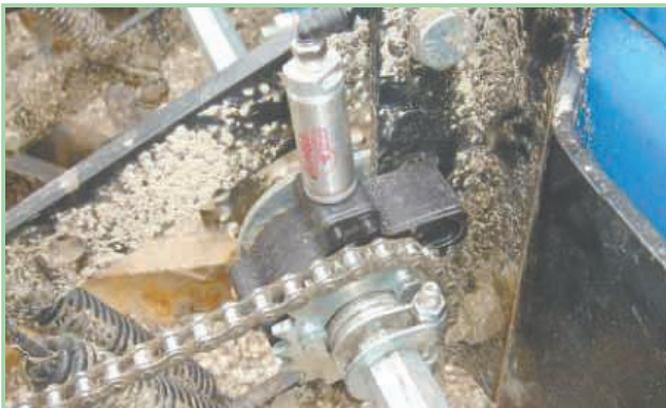
Tru Count air clutch installed on a typical chain-drive planter row unit. No planter modification is required.
