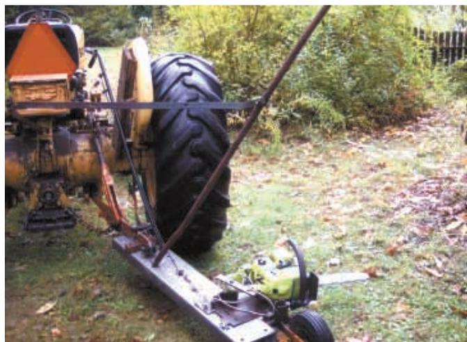
Tractor-mounted chainsaw mounts on a steel plate at rear of tractor. Once the chainsaw is running, Rechlin uses a cable to control the throttle from the tractor seat.
