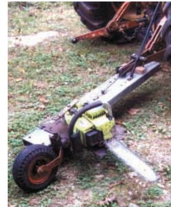
A hand-operated lever is used to swivel the chainsaw and the plate against tree trunks.
