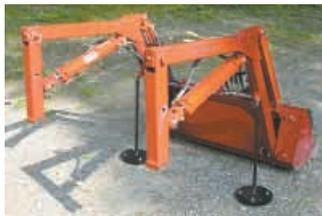
Loader quickly hooks up to a subframe that's permanently attached to tractor. The leg mounts for the loader are similar to Kubota mounts.
