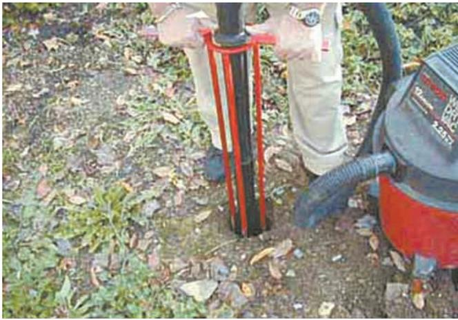
Rubber-handled grips at top of frame let operator drive chiseled steel tines into the ground. Shop vac extension tube goes down the center.
