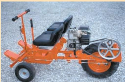
Rear-drive 3-wheeler is powered by a 5 hp Briggs & Stratton engine. The driveshaft chain-drives the rear axle.
