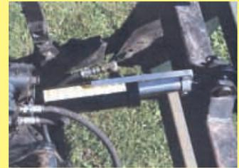
Hydraulic-operated top link has a decal with ruler marks on top that makes it easy to set implement depth.
