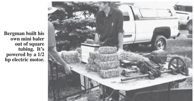
Bergman built his own mini baler out of square tubing. It's powered by a 1/2 hp electric motor.
