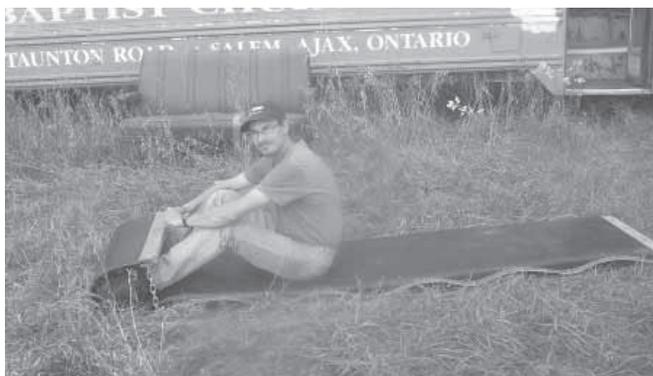
Home-built plastic toboggan is made from 3/4-in. thick plastic that's curled up on front.
