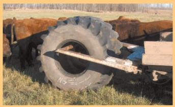
A 5-ft. section of drill stem goes through center of tire to serve as an axle.
