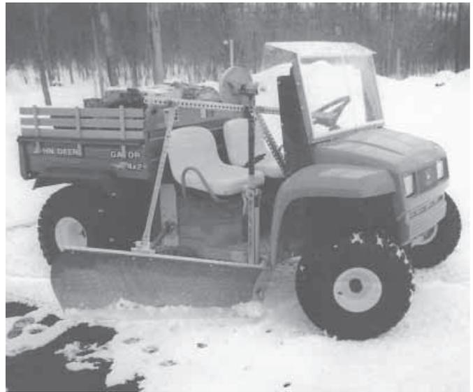
Side-mounted blade is operated by two hand controls, both located at floor level in front of passenger seat. Home-built plastic windshield extends over the dash.
