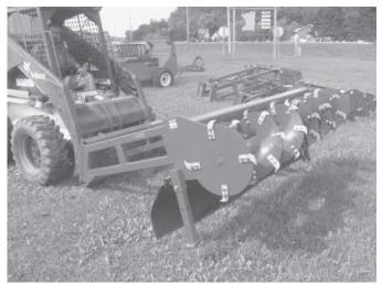
"The secret to the smooth cut is the hooked teeth on the auger," says the manufacturer of this new bunker silage facer. Auger measures 86 in. wide.
