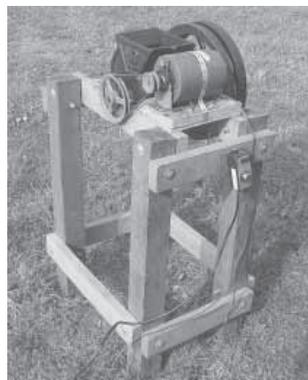
Apple grinder's drum is belt-driven by an electric motor.
