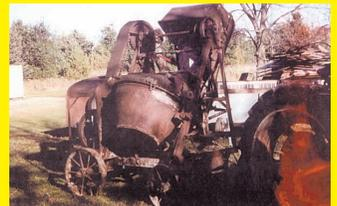
We restored a badly rusted 1920's Jaeger cement mixer to like-new condition. It rides on four steel wheels and uses an engine to chain-drive a drum on one side of the machine and a "skip" bucket on the other side. The machine was built by the Jaeger Machine Co. of Columbus, Ohio.
