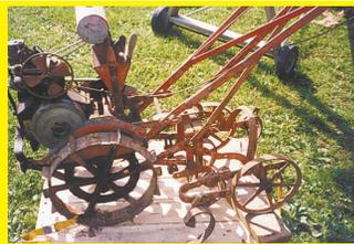
I recently restored this old Bolens 1-row garden cultivator equipped with a Briggs & Stratton gas engine. The engine still runs, and I know it's very rare. It's a "P" series engine that was built sometime between 1920 and 1923. However, I can't read the entire serial number on the engine, and no one seems to have any information on it. All the company can tell me is that I have a rare engine. The engine has no cowl-
