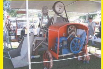
which is down on the ground. When the mix is complete in the drum, you hand crank the drum to dump it and then send the skip up with another load.
