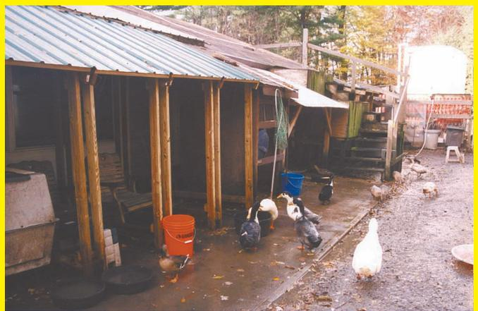
A couple years ago snow sliding off our metal roof completely blocked the back door. I designed 5 small portable lean-to's with 2 by 4 frames and metal tops that can be snugged up under the back roof of the house. Snow comes off the roof, onto the lean-to's and down to the ground. We actually put some heated
