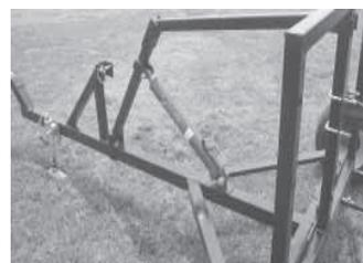
Hand-operated, 8-ton jack is used to tip the hinged frame forward or back.
