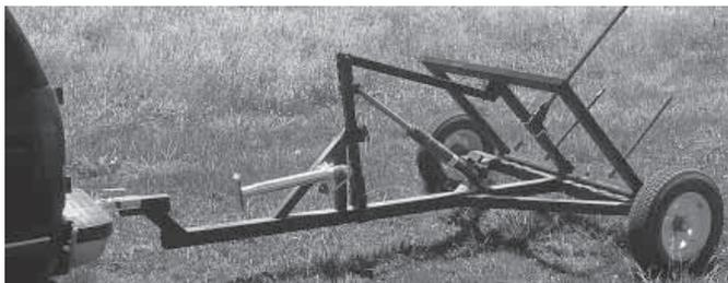
Bale hauler can be pulled by a small pickup or mini van. Bale is held at a 45 degree angle during transport.
