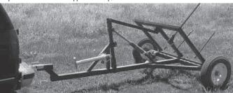
Bale hauler can be pulled by a small pickup or mini van. Bale is held at a 45 degree angle during transport.
