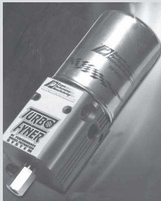
**TurboFyner filter for diesel engines also separates out water and heats the fuel before it enters the engine. It plumbs in ahead of the existing filter.**
