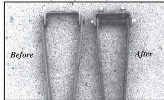
problem is that when the rivets wear out, the piece the arm pivots on also wears out. Replacing the rivets and this piece costs about \$16 per arm.
