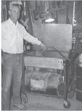
bought. He used a salvaged kitchen sink from a school cafeteria with a flip down cover made from a sheet of stainless steel. The hinged lid drops down quickly in case of a flash fire. Bugger had experience with such a fire when a magneto he was working on emitted a spark and set off a fire. Washing solvent is stored in a barrel below. To circulate it, he uses a car power steering pump. It's belt-driven by an electric motor. The washing nozzle is made from thin gauge copper tubing.
