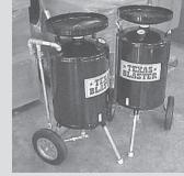
Texas Blaster has a 14-gal. tank and an easy-pour funnel for fast loading. It'll blast for 1 1/2 hours on a tank of sand.
