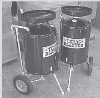
**Texas Blaster has a 14-gal. tank and an easy-pour funnel for fast loading. It'll blast for 1 1/2 hours on a tank of sand.**
