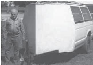
A.G. Bagwell built this trailer out of an old Dodge Grand Caravan. It has an aerodynamic, V-shaped front end which makes it easy to pull behind almost any car.
