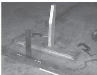
Just two parts are added to hoist - a short floor board that clamps on between boom's horizontal legs; and a longer 7-ft. 8-in. board that attaches to boom and is free to swivel on it.
