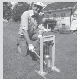
Flattener consists of a 20-ton jack mounted inside a heavy steel frame.
