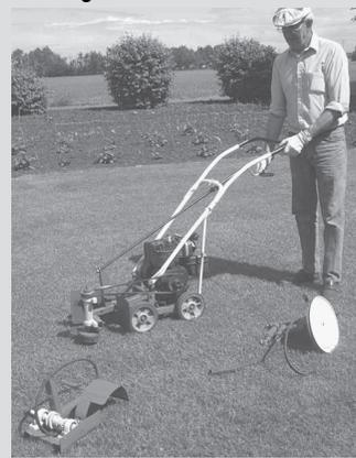
"Three-in-one" invention consists of three belt-driven attachments - a lawn edger, weed whip, and water pump.
