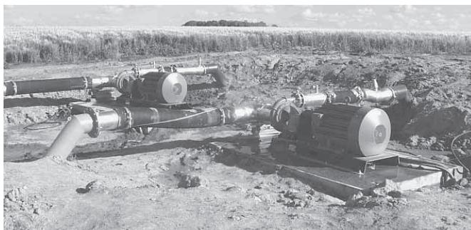
With Written-Pole motors, you can produce 15 to 75 hp on lines that were previously limited to 15 hp motors or less.
