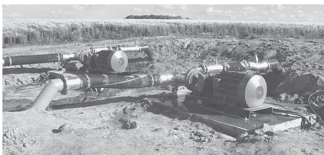
With Written-Pole motors, you can produce 15 to 75 hp on lines that were previously limited to 15 hp motors or less.
