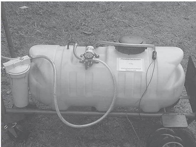
Fuel-processing system is based on technology developed by the military 60 years ago. The unit shown above produces 16 gal. of fuel per hour and is small enough to fit in the trunk of a car.
