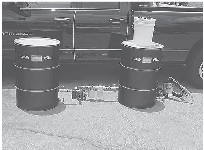
This is the larger system which processes 200 gal. of fuel every 12 to 15 min. In both systems, a mix of oil and diesel fuel passes through a set of filters and stainless steel plates.
