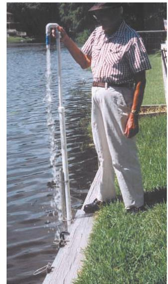
Simple emergency pump costs no more than \$25 to make, using materials that are easily obtained from any plumbing or hardware store.
