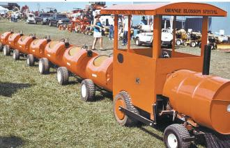
"Parade train" consists of a locomotive and seven cars made from plastic 55-gal. barrels, all painted Allis Chalmers orange. It was built by Jim Polacek of Phillips, Wis.
