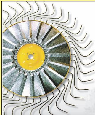
Rake teeth are individually bolted to the reel for fast replacement.
