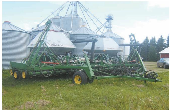
Tom McMillan wanted to apply all his fertilizer at once, as dry product, with one machine. To accomplish that, he replaced the original seed and fertilizer boxes on his Deere 752 no-till drill with two used 110-bu. tanks off a Flexi-coil air seeder.
