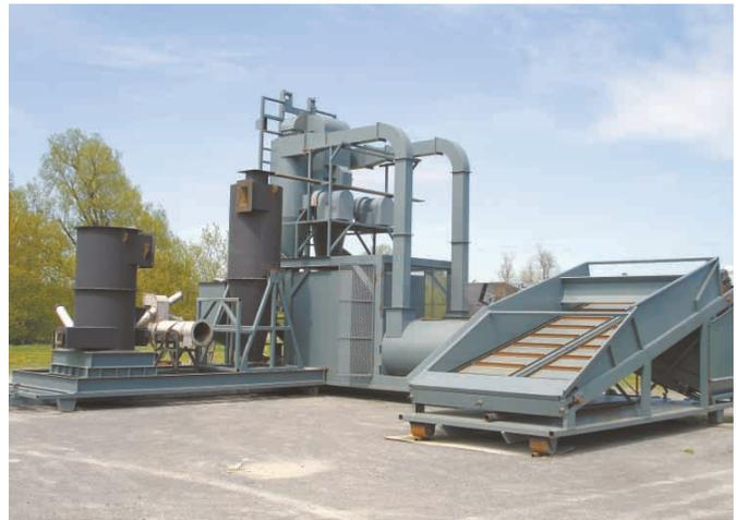
System is designed to extract oil from biomass such as chicken manure or waste wood, at the same time producing a beneficial fertilizer product. It works by vaporizing and condensing the biomass in the absence of air.
