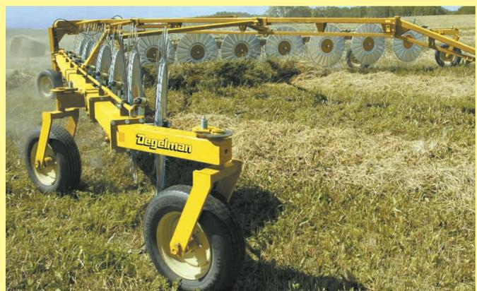
High-capacity wheel rake has oversized wheels and an overall beefier frame.
