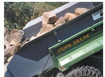
Slip-in "big box" is designed for Deere Gators and other ATV utility vehicles. The 30 cu. ft. box simply slips into the utility vehicle box with no holes to drill.
