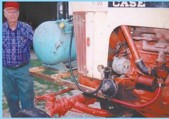
Charley Marley converted his Case 830 65 hp tractor to run on propane, using a gas controller that burns propane from a 30-gal. tank he mounted on front of the tractor.
