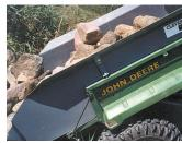
Slip-in "big box" is designed for Deere Gators and other ATV utility vehicles. The 30 cu. ft. box simply slips into the utility vehicle box with no holes to drill.
