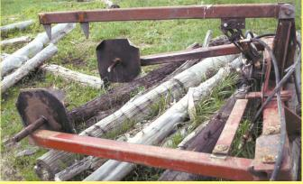
Ed Schroeder added a home-built "brake" arm to the center of his 3-pt. mounted bale unroller. It hooks up to the 3-pt. top link.
