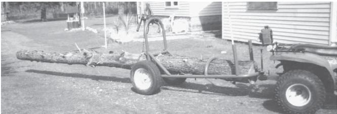
Wood hauler can be used to transport a single log up to 23 ft. long and 16 in. in diameter.
