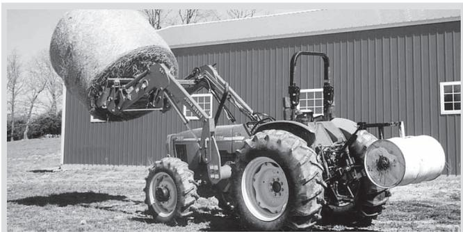
Drum improves stability when Murphy uses tractor to move 5 by 6-ft. round bales.
