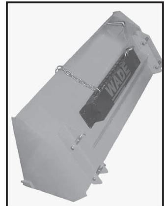
"Chain Box" on back of loader bucket provides the convenience of always having chain with you.
