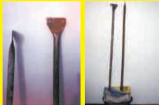
This handy scraper gets used a lot around our place. It's made from a piece of steel tubing and a used sickle blade. I just cut a V-notch in the end of the pipe, insert the blade, pinch the ends together and weld it in place. It's a tough scraper that works great for scraping manure. **(Elmer Grossen, Hillsboro, Ore.)**
