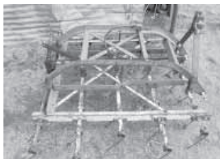
Galen Mommens built an adjustable 60-in. wide cultivator using salvaged tines from an old field cultivator (above left). He modified an old four-gang, horse drawn disk into an 8-ft. wide, 3-pt. hitch model (above right). A 6-ft. tine harrow (below left) mounts on 3-pt. hitch as does a 5-ft. wide section from an old rotary hoe (below right).
