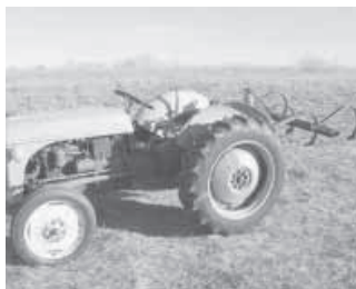
Galen Mommens built an adjustable 60-in. wide cultivator using salvaged tines from an old field cultivator (above left). He modified an old four-gang, horse drawn disk into an 8-ft. wide, 3-pt. hitch model (above right). A 6-ft. tine harrow (below left) mounts on 3-pt. hitch as does a 5-ft. wide section from an old rotary hoe (below right).
