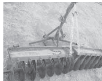
Galen Mommens built an adjustable 60-in. wide cultivator using salvaged tines from an old field cultivator (above left). He modified an old four-gang, horse drawn disk into an 8-ft. wide, 3-pt. hitch model (above right). A 6-ft. tine harrow (below left) mounts on 3-pt. hitch as does a 5-ft. wide section from an old rotary hoe (below right).
