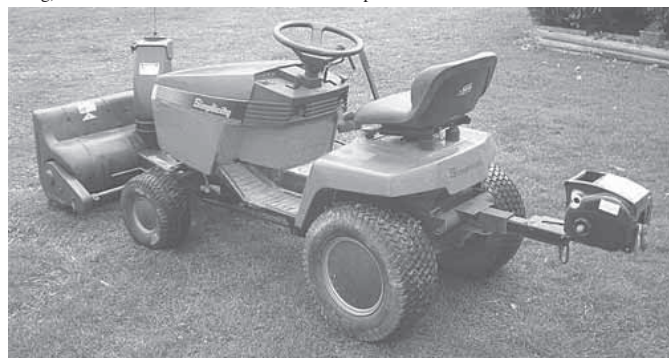
Albert Canady made this frame for his lawn tractor to support a Reese hitch. It lets him use the same attachments he uses on his truck.
