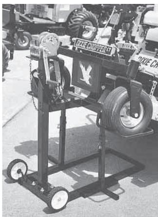
Mo-Jack's self-braking winch lifts the mower on a T-shaped lift bar that supports the front wheels.
