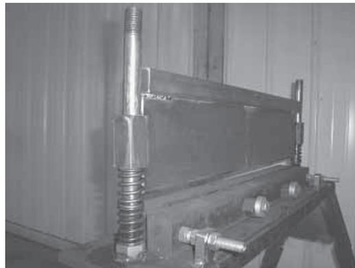
Home-built hydraulic shop press allows bending sheet metal into square tubes.
